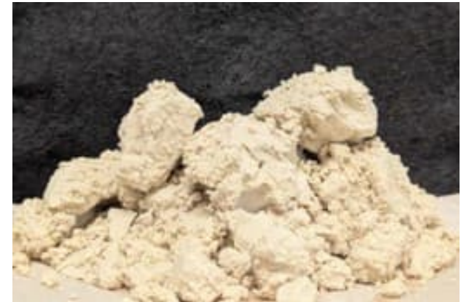
Recycled lime sludge as chemical stabilizer (ground improvement)
