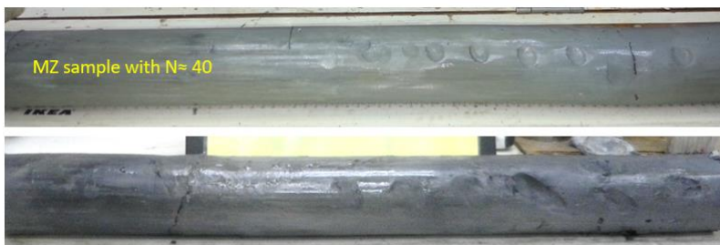
Fig. 22 Mazier samples from Jurong Formation after extrusion
