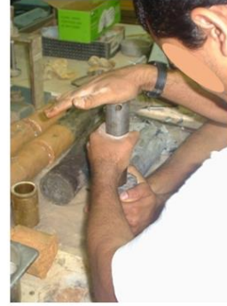
(b) Trimming using a 38mm tube
