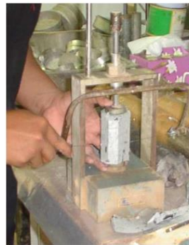
(a) Trimming using piano wire
