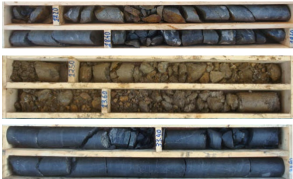
Sericite schists: during investigation and during tunnel excavation
